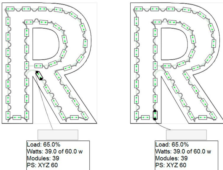
You'll notice that the wires now have a heavier stroke, and that indicates that the modules are connected to a power supply. You can think of it as the wires are now "live." There is also a connecting wire from the end of this run to the power supply.
