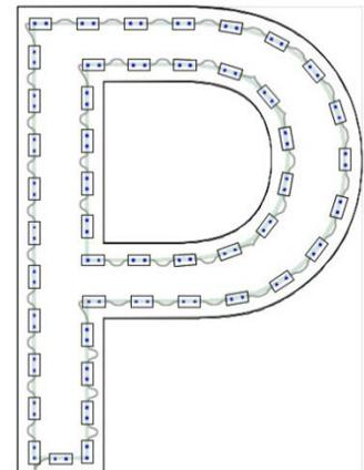
One quick note before we continue: in addition to the realistic module drawings, there are also realistic wire drawings. These wires will indicate if your modules are too far apart by switching to red. Here we have moved a module to the right, creating a section that doesn't reach, and so the wire has turned red. This provides a very quick way to see if any modules need adjusting due to wire spacing.
