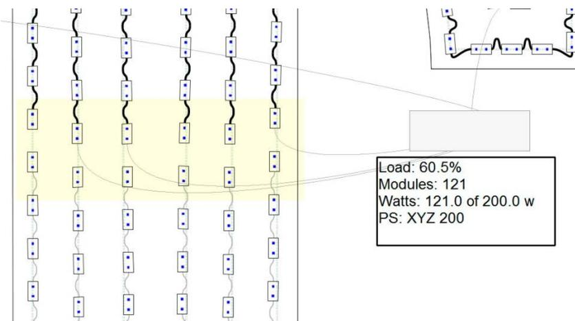
You can see in the close up image that the runs have been broken at that spot. Now you just do the same for the bottom section, and your power supplies will be loaded. You can position the power supplies anywhere you want to in the layout.
