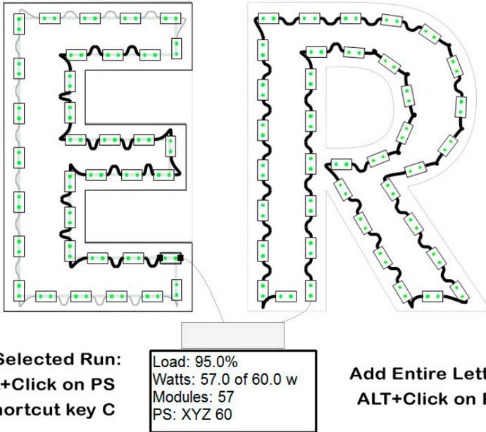
In this case the letter is populated by just one run, but if you have a letter that is populated with more than one run, such as this “E,” then you can add one run at a time. To do this, select a module in the run (it is not necessary to select the entire run), and **Shift+Click** on the power supply or use the shortcut key **C**.
