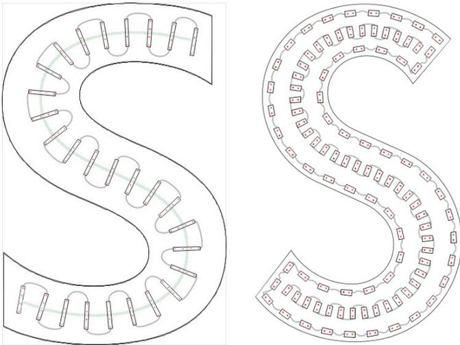
Perpendicular Alternate Rotated is a great feature that you can do in one step from a linear centerline. Keep in mind that the density commonly doubles in these cases from a linear layout, although it does depend on the module and the wire length.
