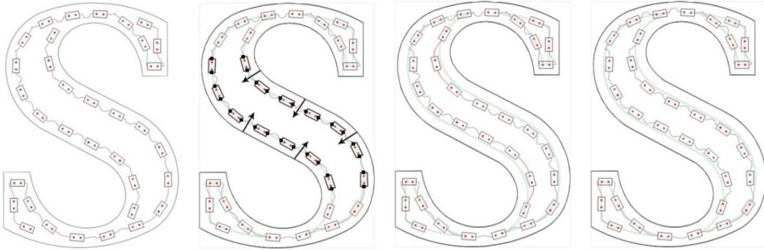
You can see the progression here in these four images. First is the original. Second shows what we want to do. Third is the initial result, but you can see that now we've created some red wires. This is due to the fact that the modules are moved away from the edge at a perpendicular from the outside angle. The result is that some modules get closer together and some get further apart. So the fourth image has the shifted sections re-spaced.
