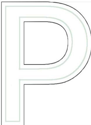
how this guide path looks, you can change one or more of the values in the property bar that we discussed above, such as Clearance or Runs, and the guide path will adjust. This letter “P” is 42” tall and has a stroke width of about 8 inches. We are going to use the XYZ Standard Blue Double module to populate with a double run. For this example, we are using **Pop: Sym**, and we get the result on the right.
