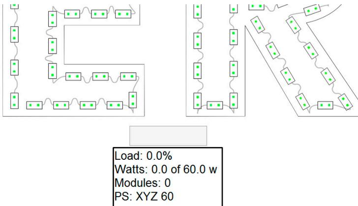
Here is the power supply that we have placed in the layout beneath the “E” and “R.” The actual power supply dimension is the rectangle on top. The larger rectangle just houses the data: **Load**, as a percentage of the total, **Watts**, as a number of the total wattage, **Modules** wired to that power supply, and **PS**, the name of the power supply.
