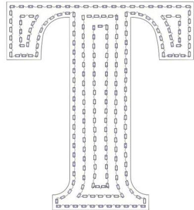
Here is a large "T" that we want to populate using two power supplies, one at the top and one at the bottom. Since this layout has runs that span the entire height of the letter, if we want to do our power supplies this way, we'll have to break several runs. Luckily the Power Supply Mode can do this for us!
