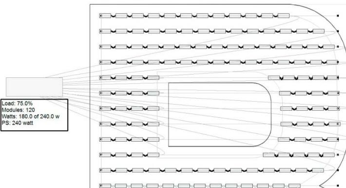
Now all you have to do is draw a box around the modules you want for the first power supply, and they will be selected, as shown here. The power supply data box will show a preview of the load for your reference, but the modules are not actually attached to that power supply yet. To do to that, go to **Power | Add Selection Rectangle Modules to Power Supply**, or use the shortcut key **B**.
